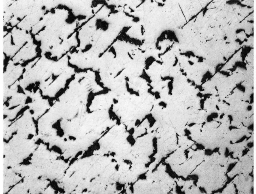
Y-2.17% H alloy ( H/Y = 1.96 ). The structure is nearly all hydride phase.
